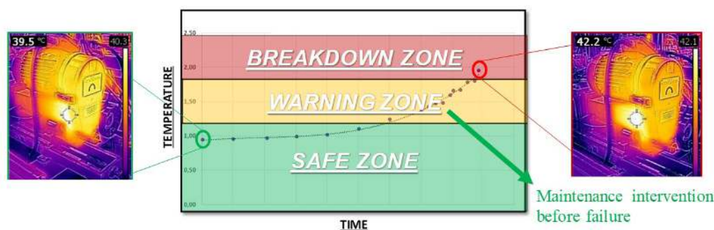
Figure 5. Maintenance policy based on the continuous condition monitoring of an operating parameter.
